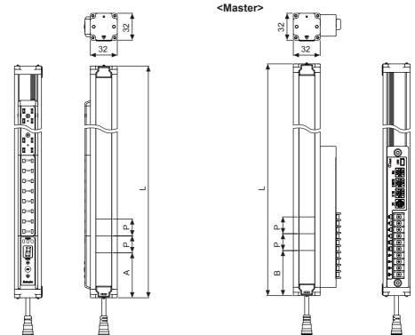
%Length of the product can be different by its ordered specification. Refer to the followings. length of the product (L) = 105+{optical axis pitch (P)×(sensing CH-1)} A: 45 to 65mm, B: 65 to 85mm
