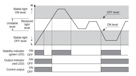
\* The waveforms of 'Operation indicator' and 'Control output' are for Dark ON. The waveforms are reversed for Light ON.
